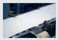
Universally adjustable infeed light barrier (IP 69K) for safe and precise product detection.
