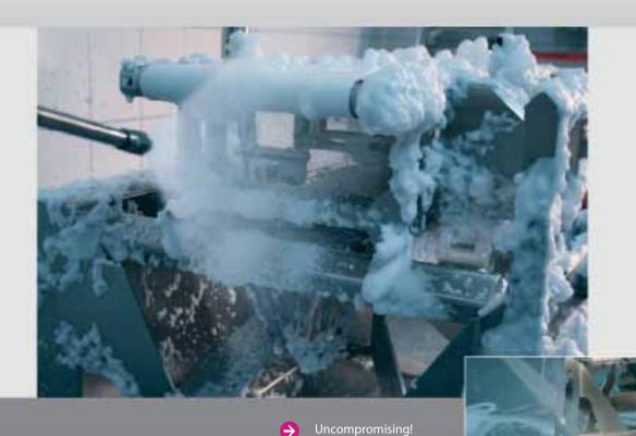
Open under frame, no hidden voids, rounded surfaces.
