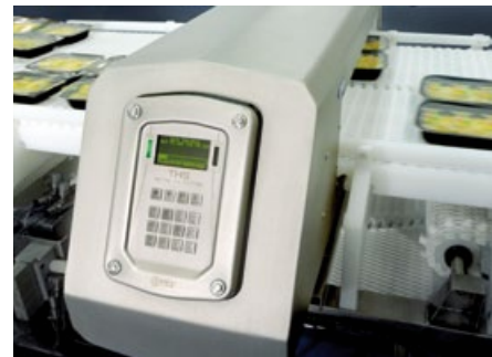
STRUCTURE AND COMPONENTS IN AISI 304 STAINLESS STEEL AND FOOD-COMPATIBLE PLASTIC PARTS (FDA, USDA COMPLIANT)
